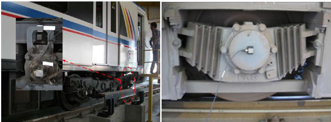
Fig. 9 Recording of vibration of rail vehicle suspension at a speed of 60 km/h [43]
